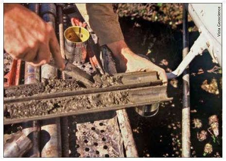
Frozen soil cores were collected in the tundra environment and were sealed in metal food-type cans on site for shipping and analysis.
