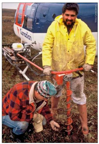
A power auger mounted on the side of the helicopter was used to collect frozen cores of the tundra. Helicopters are the only way to access the sensitive tundra environment during the summer months when the sun never sets.
