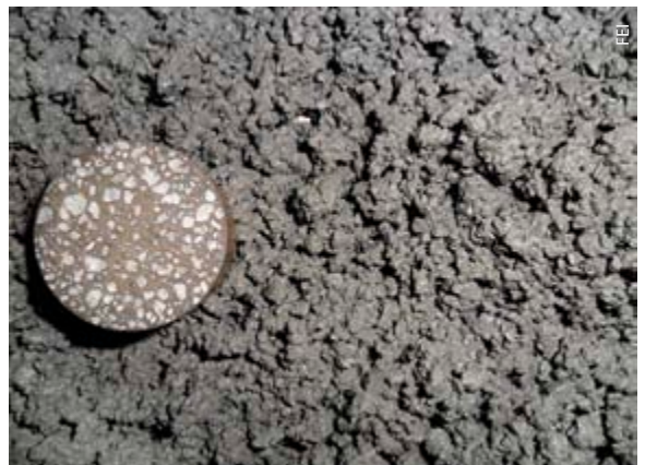
Wet cuttings sample, direct from a shale shaker, with a resin impregnated block of the same sample for comparison.
