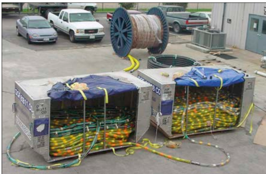
The 'staging' of a GeoStreamer prototype in 2005 used in field tests.
