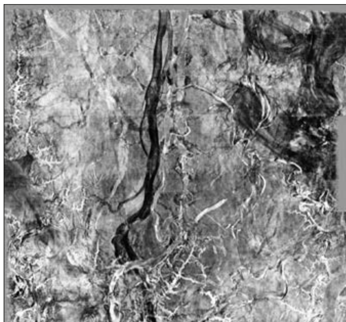
Comparison of two time slices of a region 25 km by 23 km at 120 ms TWT, corresponding to 105m depth below the sea bed. Water depth is 70m. The SWIM method applied to primary reflections (left) contains a pronounced cross-line acquisition footprint that precludes shallow geohazard interpretation. In contrast, SWIM applied to surface multiples (right) yields a remarkably continuous and high resolution final image after amplitude balancing because of the superior illumination from surface multiples. It is largely free of sail-line acquisition footprint.
