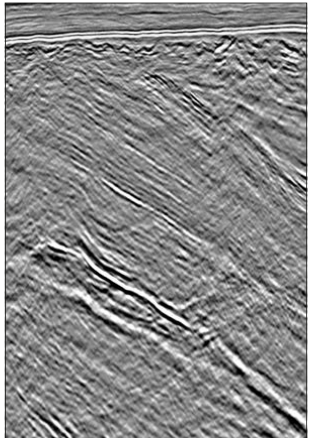
Applied Clari-Fi processing sequence enhances deeper imaging and broadens frequency content of the data
