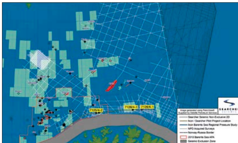
Figure 1: A series of 2D lines extending west–east towards the Norway/Russian boundary. These data have recently been derived by Searcher Seismic, Perth, as part of an acquisition process in the Barents Sea in 2013.
