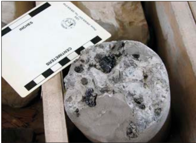
Figure 4. Bitumen in vuggy crystalline dolomite core at a depth of 478m in well RH-2 (Wadi EsSir Formation, Upper Cretaceous). Photograph by Mark Fitzpatrick in Naylor et al., 2013, with the authors' permission.
