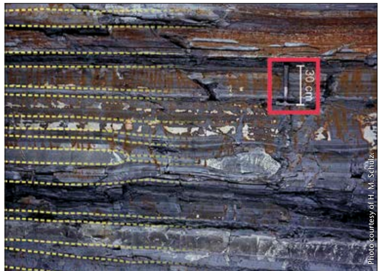
Figure 2. Jurassic Posidonia shale – typical of what shales often look like. Small scale vertical heterogeneities, as visualized with the yellow broken lines in the left of the photo, indicate variable depositional conditions and hence, likely variability in organic matter contents and preservation.
