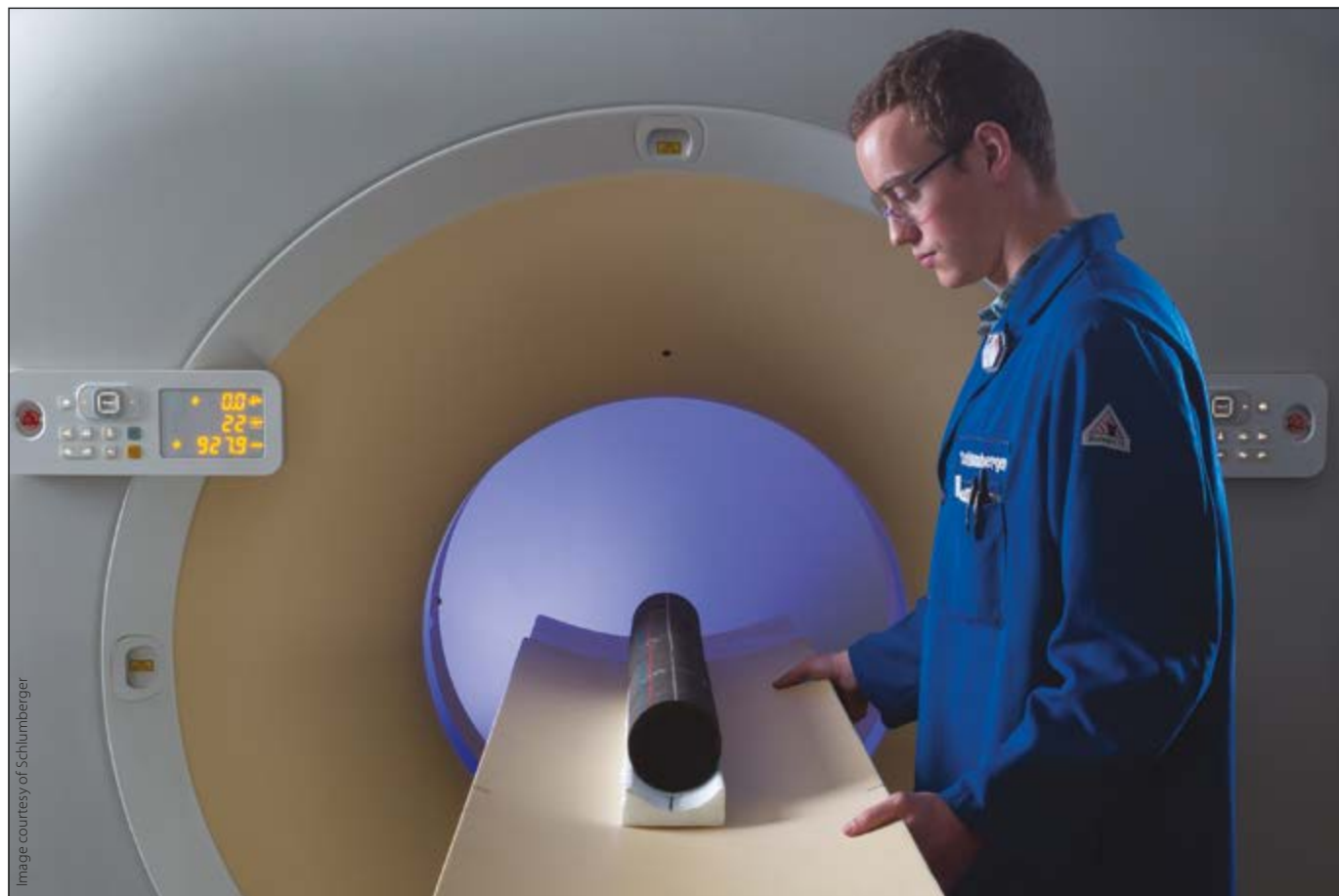
A whole-core sample is positioned for CT imaging using a dual-energy multislice scanner – the start of the process.
