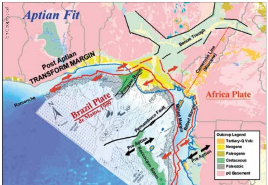
Figure 1: Tectonic map showing the restored fit of the Brazilian plate at Aptian time. Surface geology shown on the African plate, major Cretaceous rift basins and break-up direction shown.
