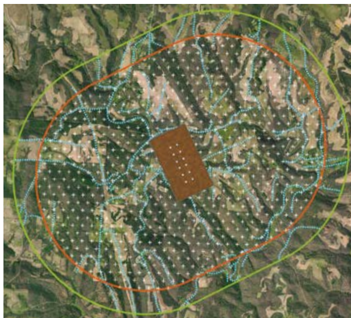
3D design to image 12 planned Utica wells from a pad in Eastern Ohio. Vibroseis source positions are confined to roads to optimize acquisition efficiency. Receiver positions are evenly distributed in a hex array using AutoSeis® recording nodes.
