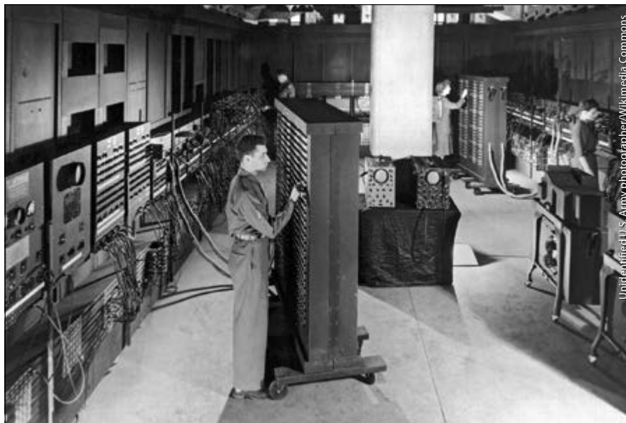
Installed in 1945 at the Moore School of Electrical Engineering, University of Pennsylvania, USA, ENIAC contained more than 100,000 components and weighed approximately 30 tons. It was the first programmable general-purpose electronic digital computer. The first test problem run consisted of computations for the hydrogen bomb.
