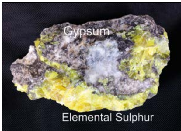
Organic-inorganic interactions in pore water – TSR. Solid TSR products are composed of calcite and elemental sulphur, both formed by aqueous dissolution of anhydrite.
