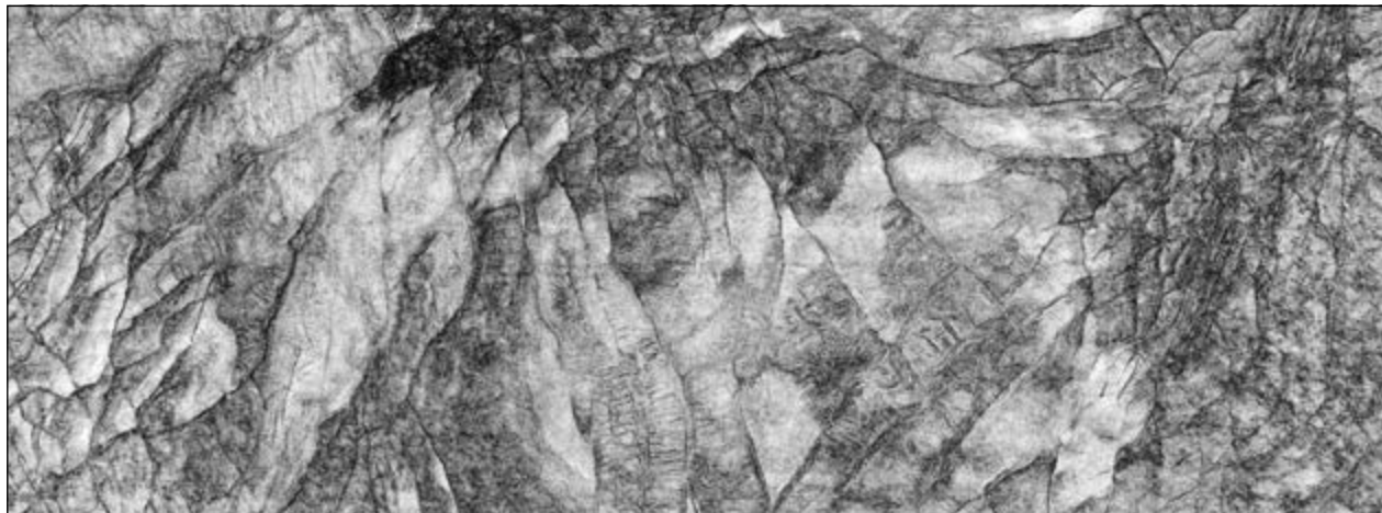
Incoherency plot showing the extent of faulting affecting the Jurassic sequence at 3.5 sec TWT in the Northern Carnarvon Basin.
