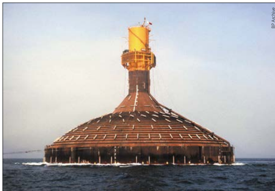
Dubai Khazzan No.1 being towed to its site in the Fateh oilfield in August 1969.
