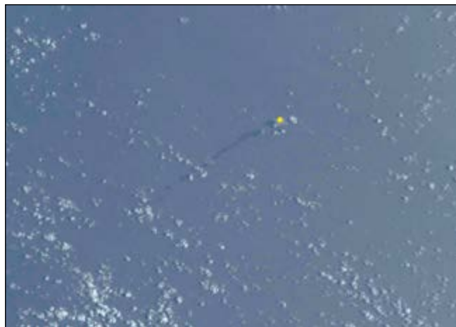
Oil slick from an active oil seep thought to be located directly over toe-thrust structures offshore Somalia.
