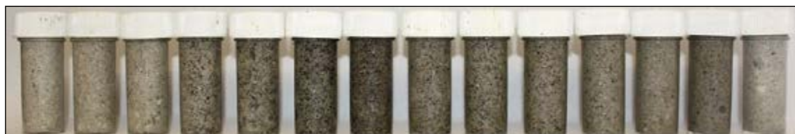
Figure 2: Wet cuttings through an oil-stained reservoir (note increase then decrease in color corresponding to oil concentration).
