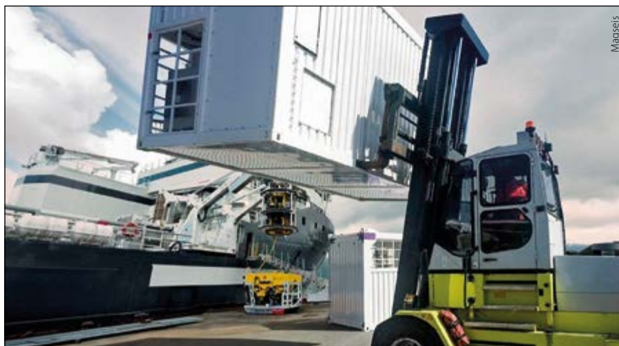
The modular MASS being lifted onboard, with an ROV in the background, between the vessel and the truck.
