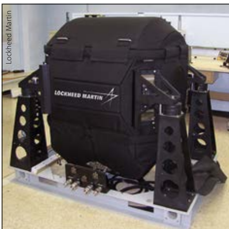
The eFTG, designed and built by Lockheed Martin Corporation
