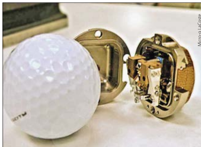
The latest generation borehole gravity sensors are smaller than a golf ball and operate in cased and uncased wells less than 3 inches in diameter.
