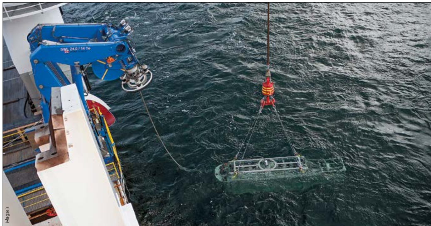
The ultra-deepwater node deployer ready to be lowered and detached from the crane, after which it will be controlled by the umbilical as it is submerged.
