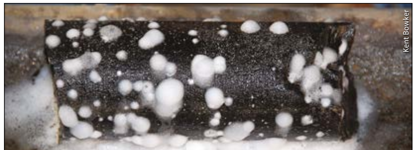
Barnett core bleeding gas, indicating a much higher gas content than studies had predicted.
