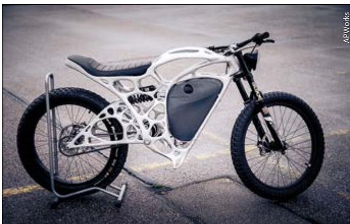
APWorks Light Rider motorcycle: 3D printed aluminium frame, 6 kw electric motor, total weight 35 kg.
