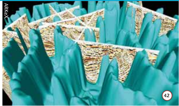
Gravity gradiometry combined with seismic data can help unravel complex geological settings.
