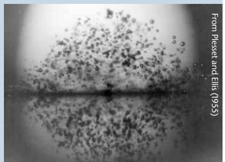
Photograph of a transient cloud of cavitation bubbles generated acoustically.
