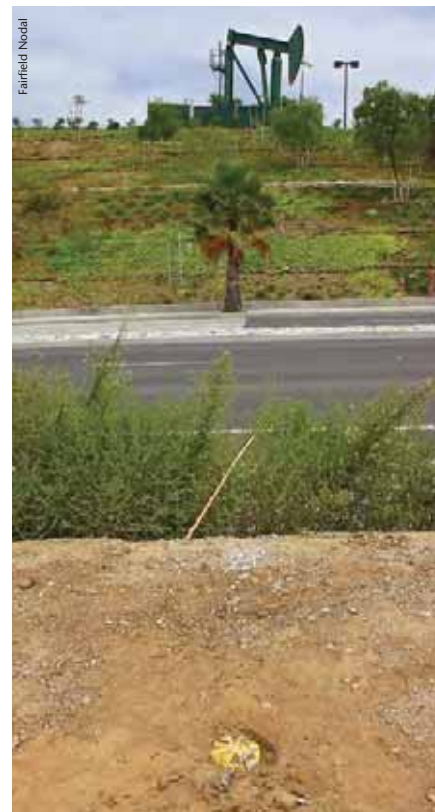
The Fairfield Nodal self-contained sensor has minimal environmental impact. It is the only truly cableless system since there are no geophone cables.
