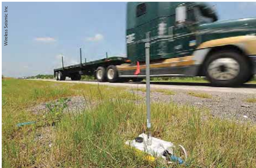
With a cabled seismic system, special protective covers are needed to cross a road, and even then, if something heavy like a truck comes along, the cable will take abuse. Rails and rivers are even more problematic. Cableless systems provide the answer.
