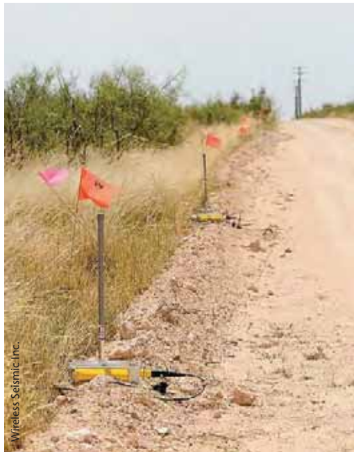
With a real time seismic system, a central control room receives all the data being collected from the cableless sensors, allowing real time quality assurance.
