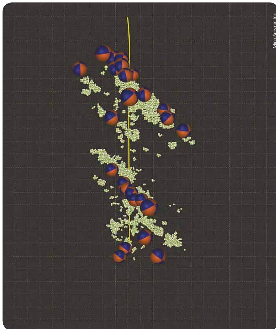
PSET® processing and imaging technology identifies source mechanisms that help geologists understand how the rock is breaking during fracturing. Operators use this information to optimize their completions and field development strategies.
