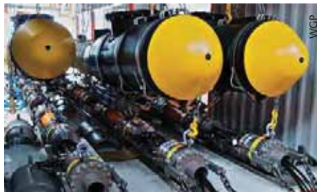
The Portable Modular Source System used by WGP on ION's Arctic exploration program
