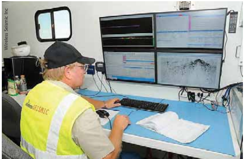
With a real time seismic system, a central control room receives all the data being collected from the cableless sensors, allowing real time quality assurance.
