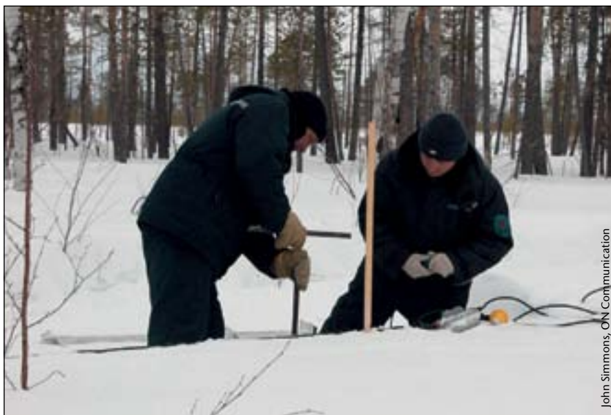
Planting 4C geophones in West Siberia. Working in the Arctic presents many challenges.
