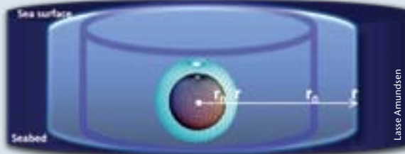
Sound generated by a sound source (shown as a white dot) at mid-depth in the ocean. At first the sound is radiated equally in all directions; sound levels then decrease rapidly with spherical spreading as sound spreads out from a sphere with a radius of r_0 to a larger sphere with a radius r . But once the sound is trapped between the top and bottom of the ocean it gradually begins to spread cylindrically, with sound radiating horizontally away from the source.
