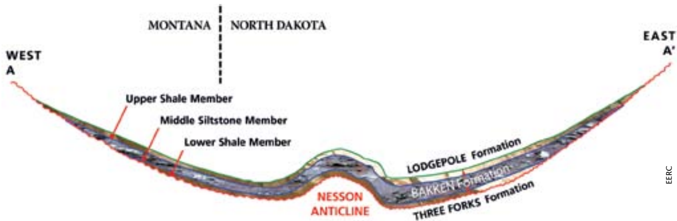
The Three Forks, Bakken, and Lodgepole formations all pinch out on the flanks of the Williston Basin.
