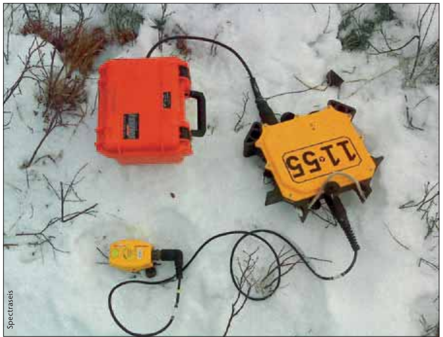
Figure 2: An UltraSense™ microseismic recording node monitors a fracture treatment in Canada.
