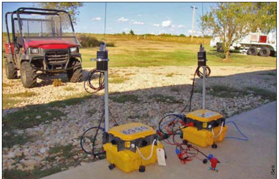
Choices in time-stamping: two Sigma units, which are receiving essential timing information via VHF synchronisation system, used when GPS signals are unavailable.
