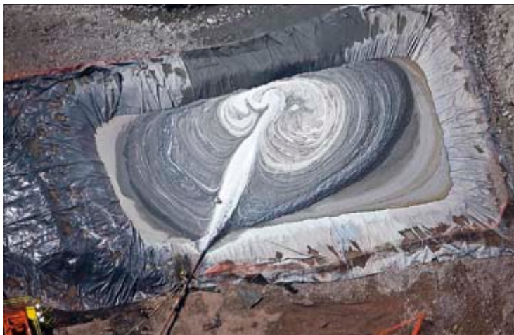
Fracture fluids are often sprayed into visqueen-lined pits (left) that can leak. The poly-asphalt containment pit (right) may cost twice that of visqueen-lined pits but provides a containment system very resistant to wear and corrosion. This pit has a grid added above it to protect wildlife.
