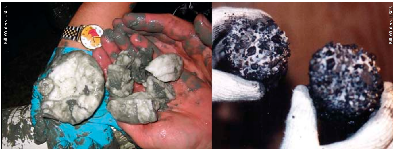
A massive hydrate layer (left) obtained from fine-grained sediment recovered in a marine setting in the Gulf of Mexico, compared to (right) hydrate recovered in a coarse-grained gravel layer from an Arctic setting, the Mallik 2L-38 well, drilled in the Northwest Territories of northern Canada.
