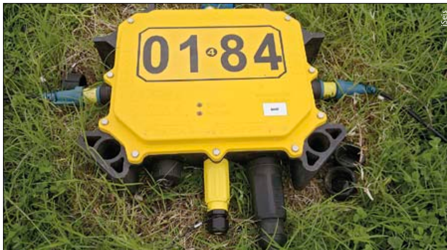
A USB (bottom of picture) actively harvesting data from a Sigma unit
