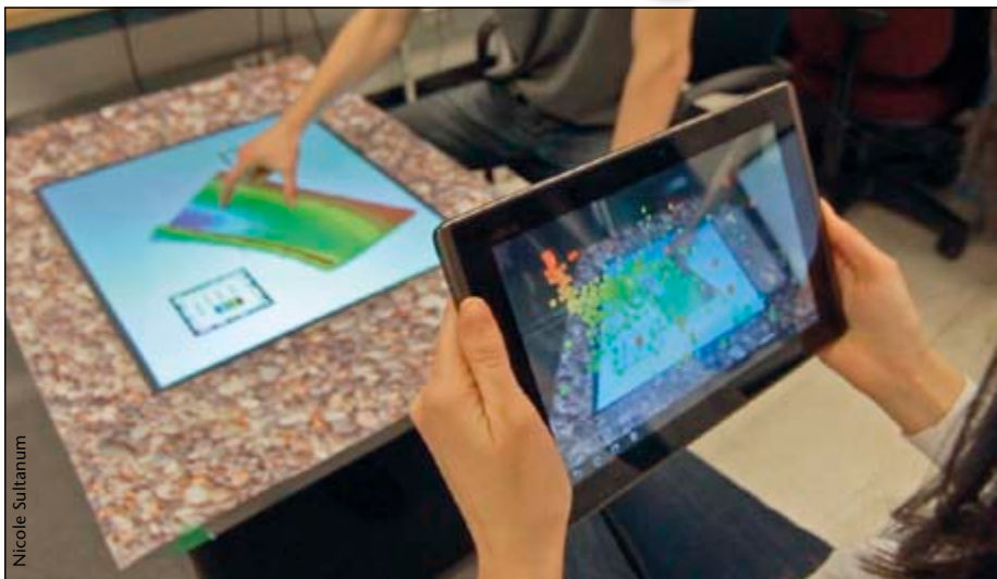
Multiple users can manipulate a point-based data set through a camera-enabled tablet.
