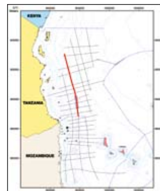
Strike line. Strike extent (> 50 km) of Early Tertiary high-amplitude, potential fan system. Note feature is encased in transparent (shaly) facies, enhancing the likelihood of a regional stratigraphic trap.
