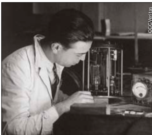
One of the first quartz seismographs, prototype PQ1, developed in 1931, one of the early advances made by seismic service companies to assist geologists in the search for hydrocarbons
