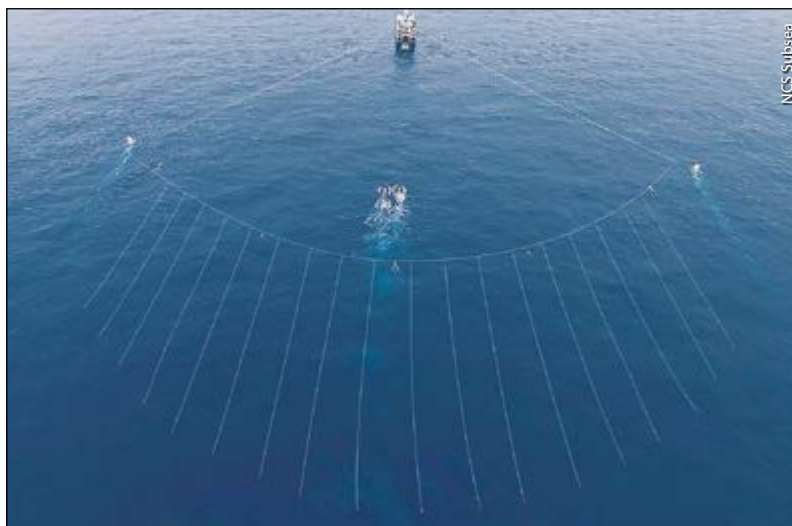
Deployed P-Cable seismic acquisition system, with 18 streamers (100m) at 12.5m spacing.
