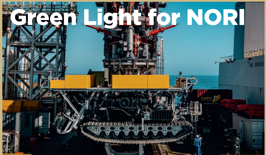
The Allseas-designed nodule collector vehicle awaiting launch.
