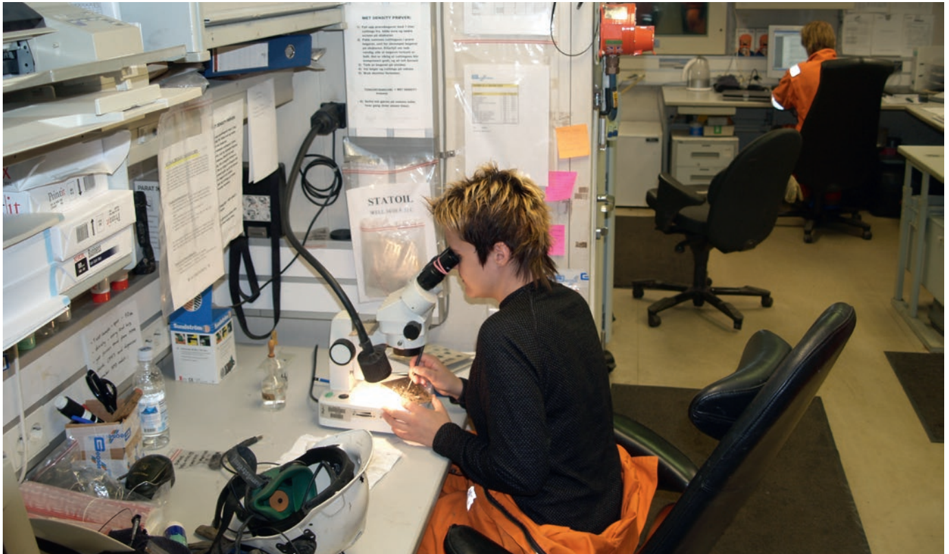
Biostratigraphers working on an offshore rig in the Northern North Sea. Micropalaeontology analysis like this allows important calibration during drilling operations to compare the pre-drill geoprognosis versus observed stratigraphic markers to safely reach the desired target and maximise reservoir contact. Palaeoenvironmental indicators can also improve understanding of the depositional system across the reservoir interval which can improve estimates of net to gross and other parameters that impact STOOIP calculations in exploration wells.
