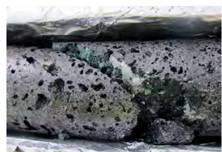
| Precipitated carbonates in cored basalt from the Carbflix CO 2 injection site.
