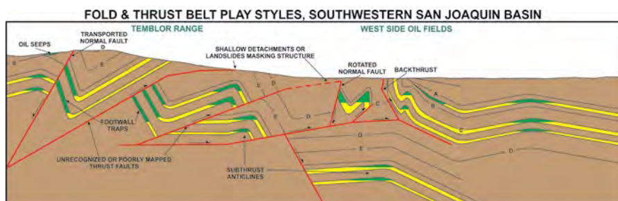
Figure 2: Diagrammatic cross-section showing the various oil trapping mechanisms encountered in the WSFB of the SJB. Most of these traps are associated with development of the fold and thrust belt (F&TB). Underexplored and previously poorly imaged synclinal areas with sub-thrust and sub-detachment anticlinal traps are of primary interest. These areas are more extensive than previously thought and have concealed oil traps and sub-basins with known oil source and reservoir rocks (Davis et al., 1988; Davis, 2015; Davis and Namson, 2017).
