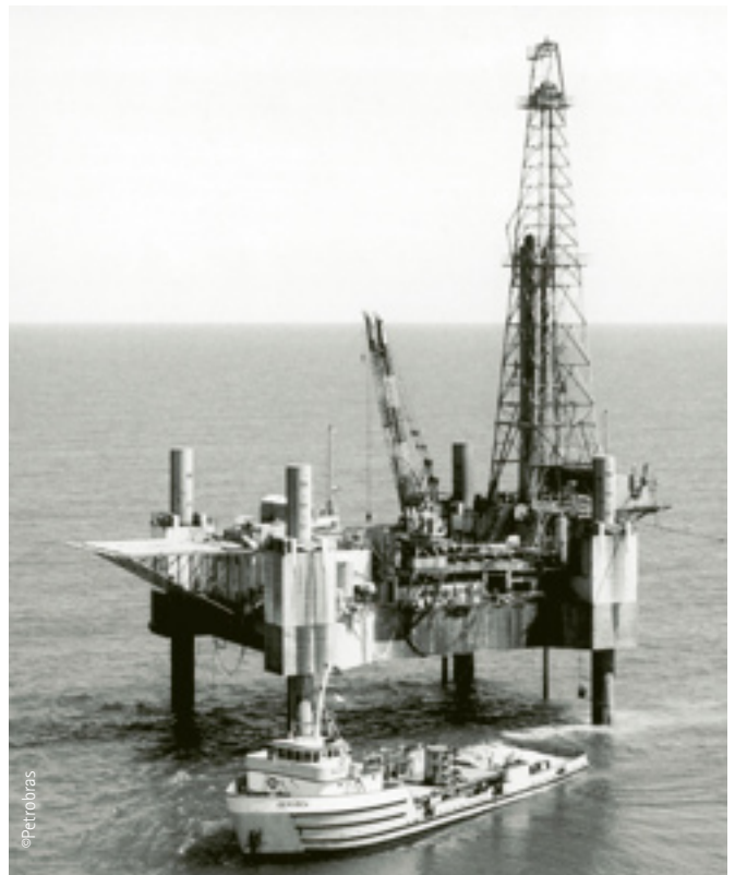
Jack-up platforms were used for the first offshore exploration offshore Brazil and account for the first discoveries. Campos basin drilling started in 1971 and the early wells were also drilled from jack-up platforms.
