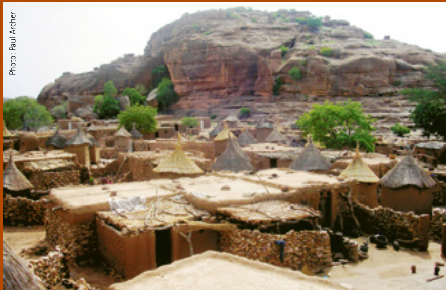
The Dogon live in mud-brick buildings, often with elaborately carved doors and shutters, in family compounds which contain granaries topped with distinctive conical straw roofs.
