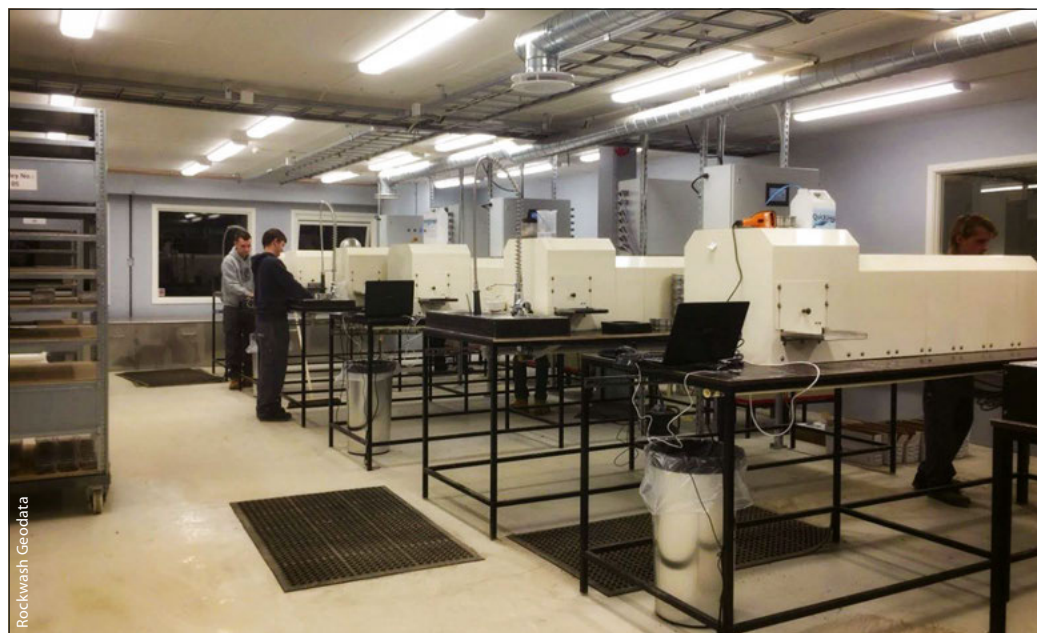
Figure 4: Rockwash machines carrying out automated washing and drying of cuttings samples for the NOROG Released Wells Initiative in Stratum Reservoir's Sandnes facility.
