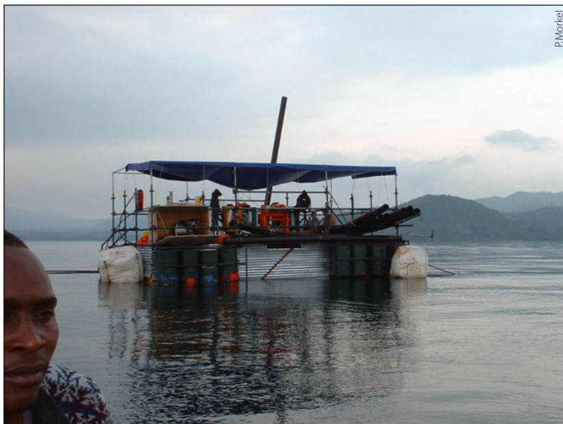
Figure 4: The test rig was cheap and ugly but was able to test gas separation to 70m depth.
